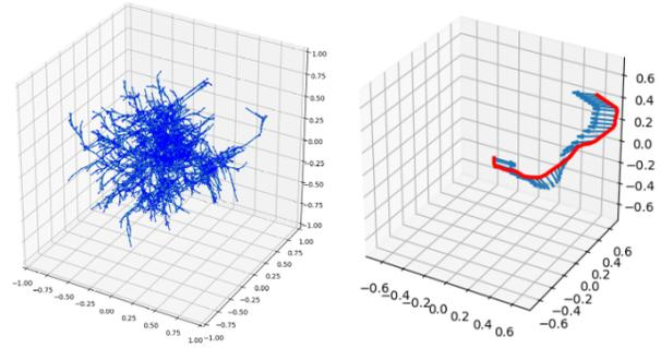
Fig. 3. RRT nodes for the rigid body dynamics (left) and a feasible solution (right).
